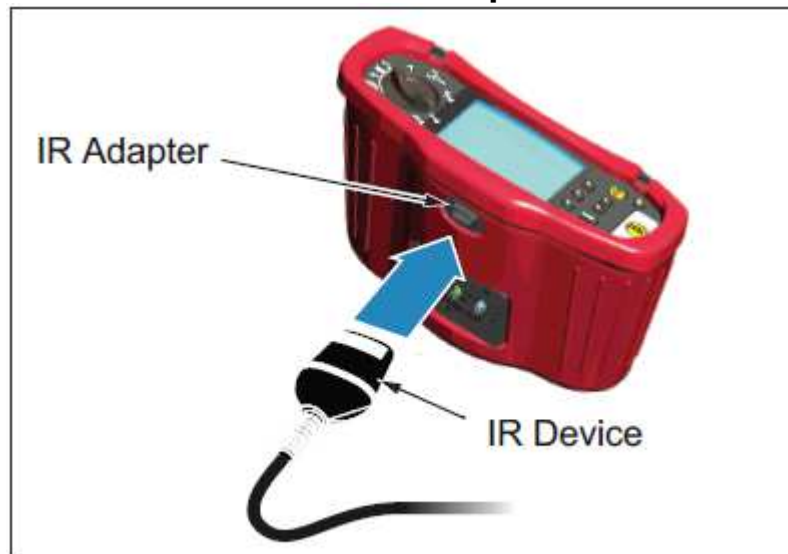
Figure 23. Attaching the IR Adapter
