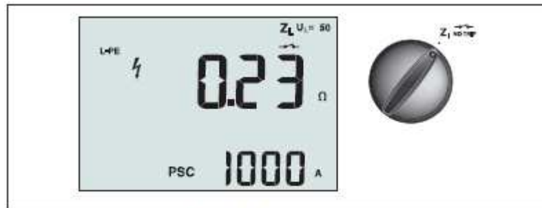
Figure 11. Loop/Line Impedance/Switch and Terminal Settings
