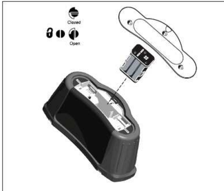
Figure 24. Replacing the Batteries
